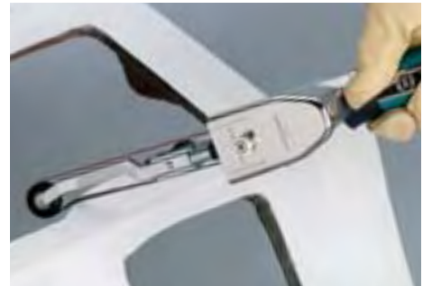
Optional offset Contact Arm allows belt to conform to a variety of contours.
