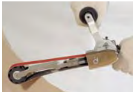
Slack sanding with optional 15375 Arm.
