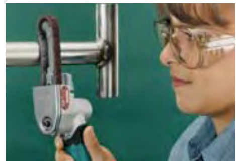
Clean and finish using non-woven nylon belts.
