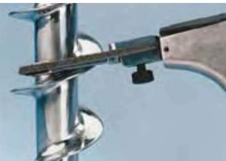
Clean and finish using non-woven nylon belts.
